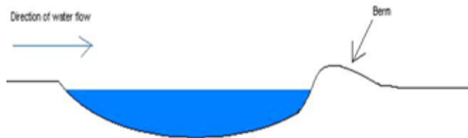
Figure 2. Water should flow into the low side of the rain garden and meet resistance to outflow by the raised berm. (Photo courtesy of Mitch Woodward, North Carolina Cooperative Extension)
